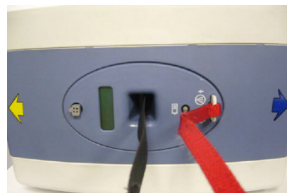
Directional arrows on underside of hoist
