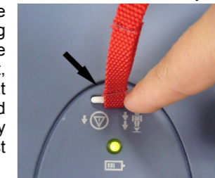
Return power to the hoist unit by pressing in the plastic tab
