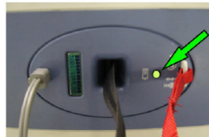
Figure 4D - Hoist ON indicator
